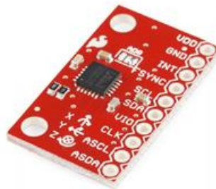
Fig 29. The Accelerometer + Gyroscope IMU MPU 6050 from DiGi
