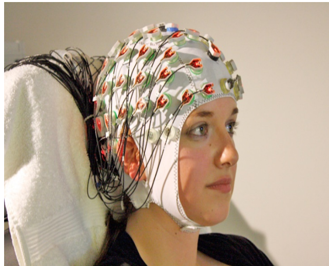
Figure 4.6. Non- invasive EEG scanning devices are mounted on caps or headbands [ME14]
